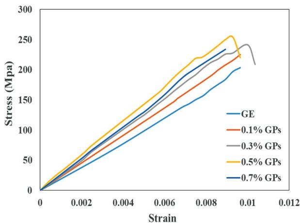
**Figure 2:** Stress-strain curves for GE and GP-GE composites under compression
