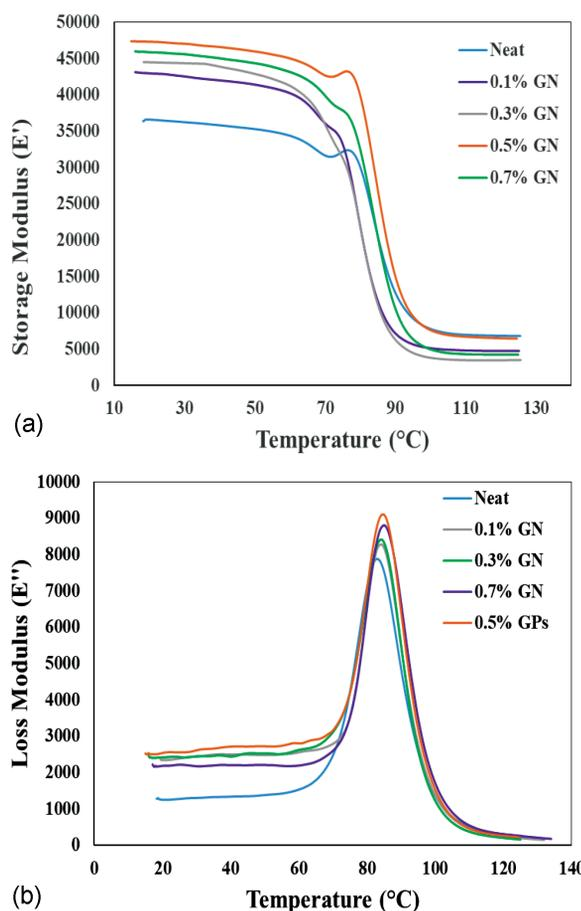
Figure 1: Storage modulus ( $E'$ ) and loss modulus ( $E''$ ) of GE and GP-GE composites
