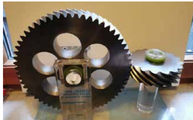
Figure 10 : A helical S-gear pair with perpendicular shafts as used in centrifuges
