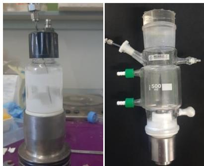
Figure 1: ultrasonic set-up for GC measurements
