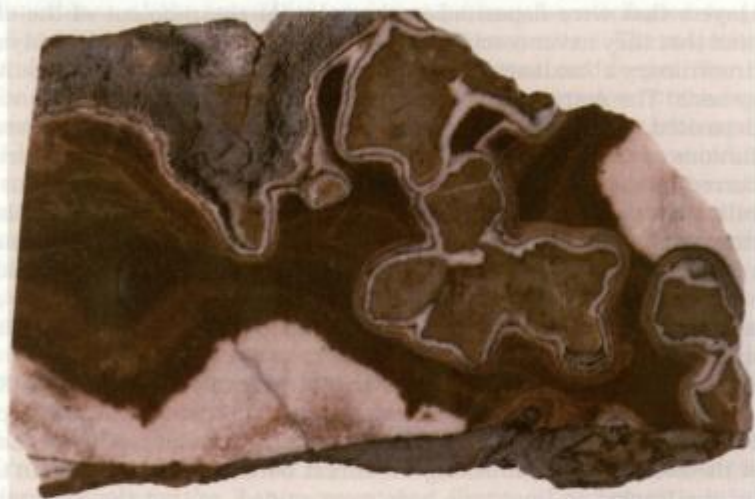
Fig. 6. A detail of the solution cavity filled by sparitic radial calcite and red carbonaceous clay; the top of Krn, natural size
