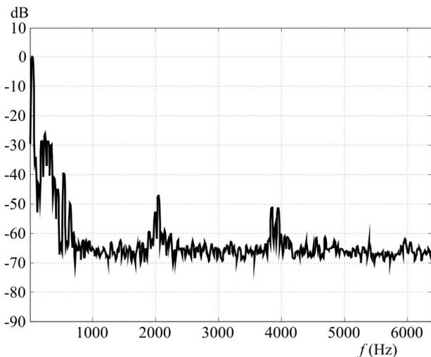
**Figure 12:** Output current spectrum with SAPF active
