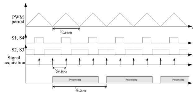
**Figure 2:** Timing diagram of sampling, switching and algorithm execution
