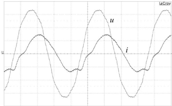
**Figure 7:** SG output voltage and load current ( $k_u = 1000\text{V/div}$ ,  $k_i = 5\text{A/div}$ ,  $k_t = 5\text{ms/div}$ ).
