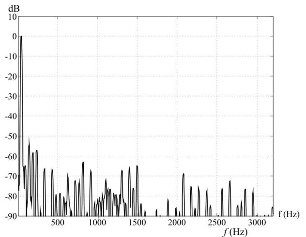
**Figure 6:** Total system voltage spectrum with SAPF active.
