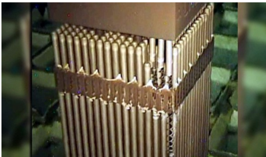
Figure 13: Damaged fuel assembly AD11 (Source: Kanal A)
