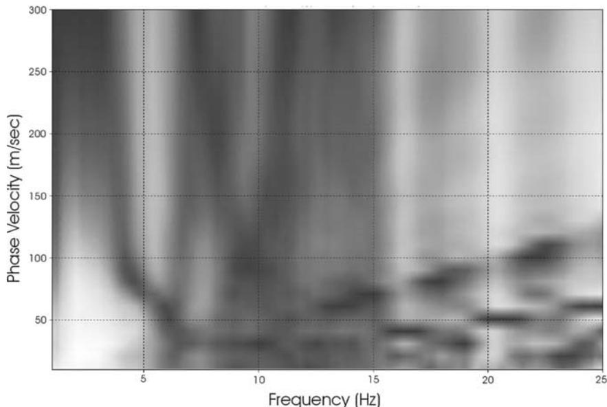
**Figure 10.** Dispersion image of passive MASW measurements
