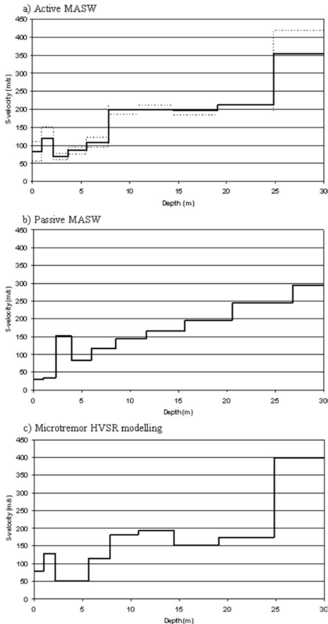
**Figure 14.** Shear-wave velocity profiles from a) active MASW (with  $\pm$  one standard deviation), b) passive MASW and c) microtremor HVSR modelling
