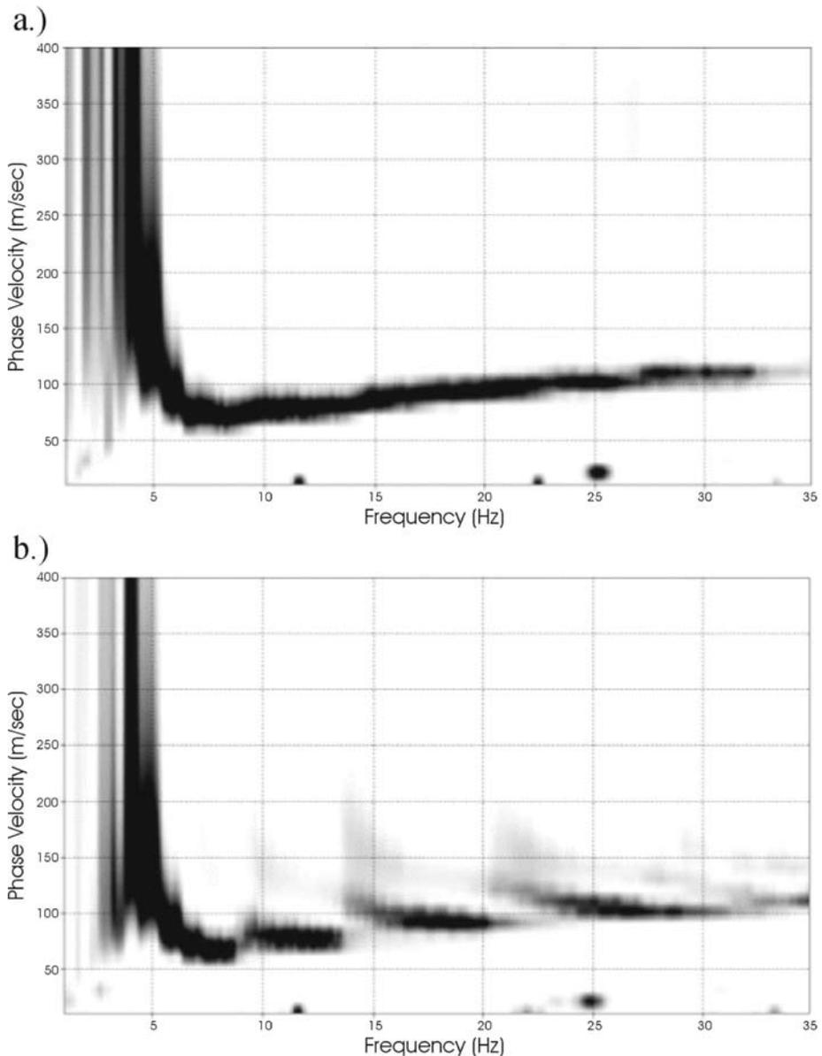
**Figure 6.** Dispersion images of two active MASW measurements: a) example with only fundamental mode of surface waves visible, b) example with higher modes of surface waves at frequencies  $\geq 8$  Hz
