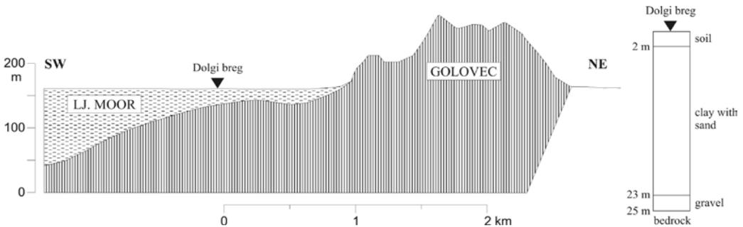
**Figure 2.** Profile across the Ljubljana Moor (Quaternary sediments) and Golovec hill (Permian and Carboniferous sandstones, conglomerates and shales) with the location of measurements at Dolgi breg
