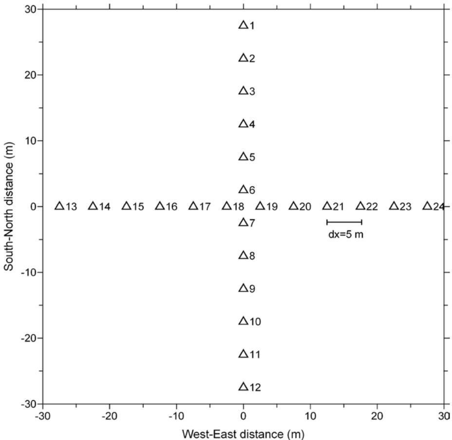
**Figure 8.** Cross geophone array used for passive MASW measurements
