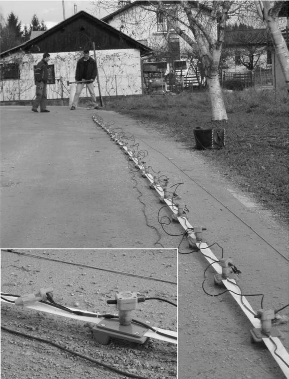
**Figure 4.** Land streamer with 24 vertical geophones and a sledgehammer as a seismic source; on a small insert a detail of geophone mount is shown
