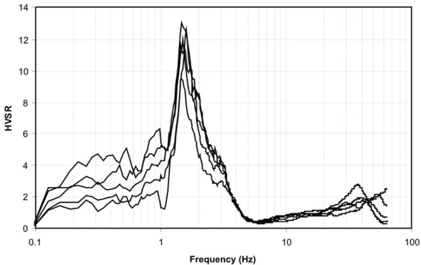
**Figure 12.** HVSr curves of five microtremor measurements
