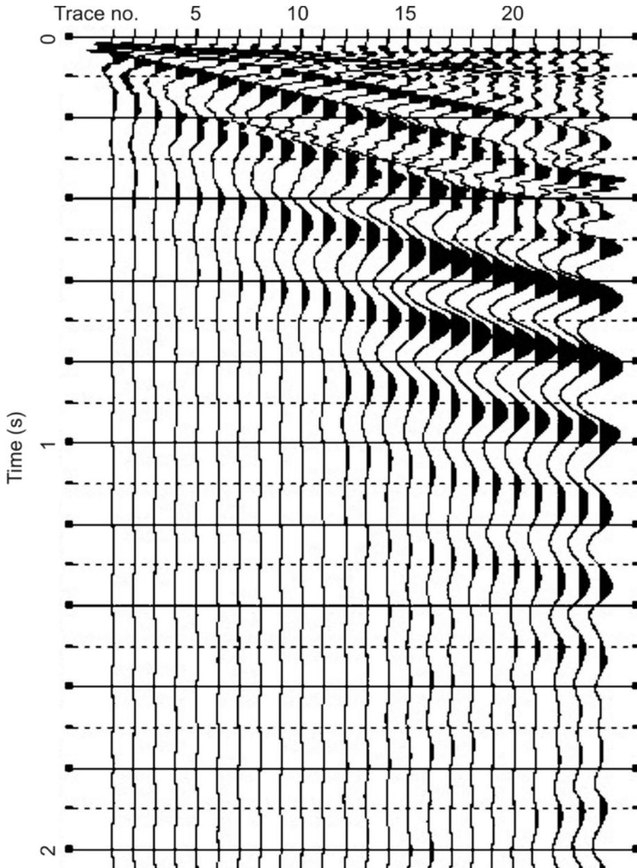
**Figure 5.** Seismogram example of active MASW measurements
