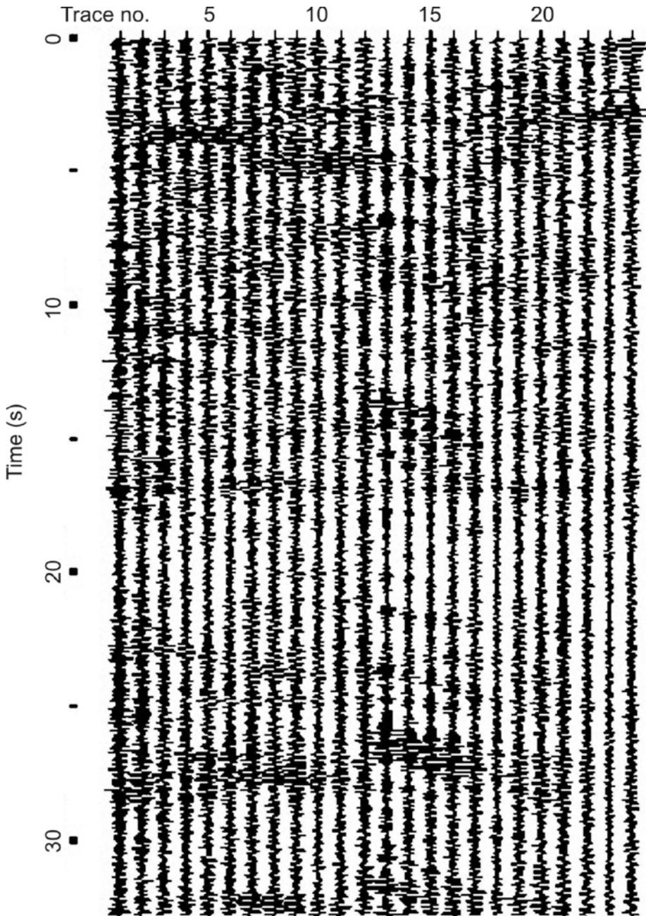
**Figure 9.** Seismogram example of passive MASW measurements
