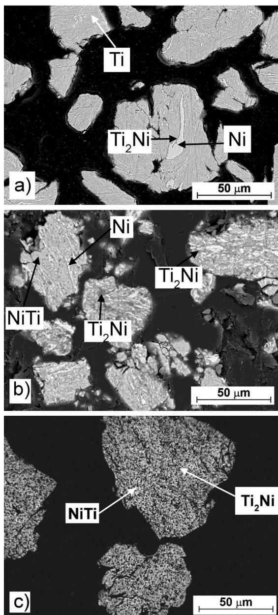
**Figure 2:** Microstructure of NiTi50 (in amount fractions, at%) alloy powder prepared by mechanical alloying for: a) 15 min, b) 45 min, c) 120 min
