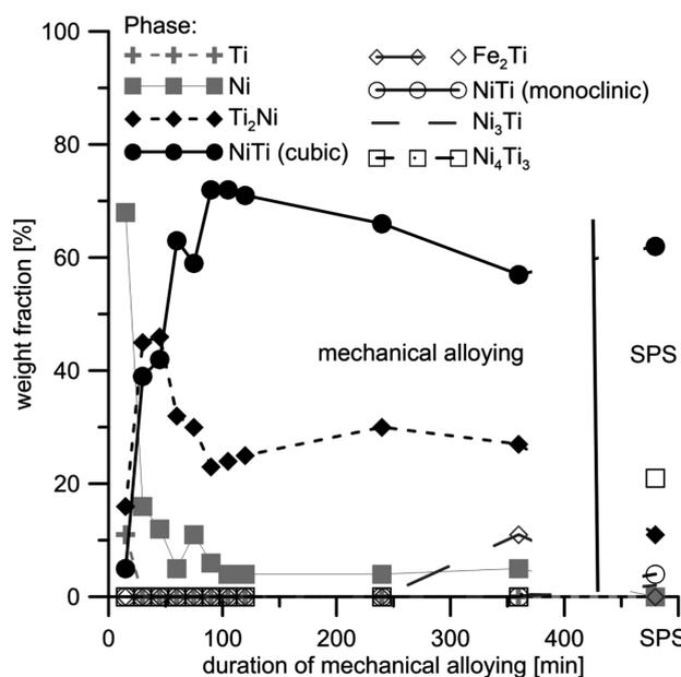
**Figure 1:** Amounts of phases in milled powders and SPS-consolidated sample (determined by XRD and Rietveld refinement)
