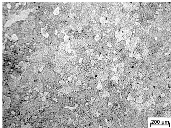
**Figure 3:** Microstructure of the NiTi alloy prepared by mechanical alloying for 120 min and spark-plasma sintering at  $900\text{ °C}$  with a heating rate of  $300\text{ °C min}^{-1}$
