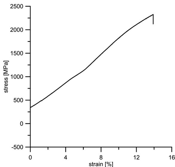
**Figure 4:** Stress-strain curve in compression of the NiTi alloy prepared by mechanical alloying for 120 min and spark-plasma sintering at  $900\text{ °C}$  with a heating rate of  $300\text{ °C min}^{-1}$
