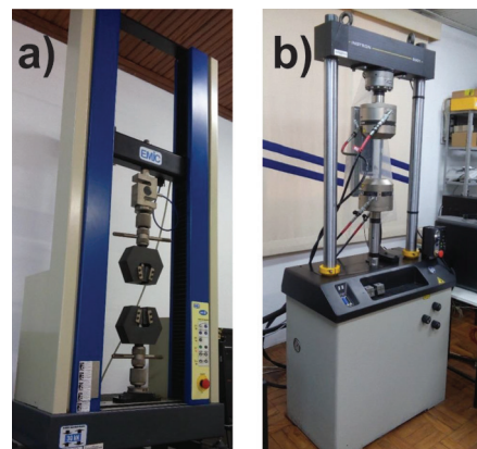
Fig. 6. Equipment used in the shear test: a) EMIC® (Machine 1) and b) Instron® (Machine 2)
