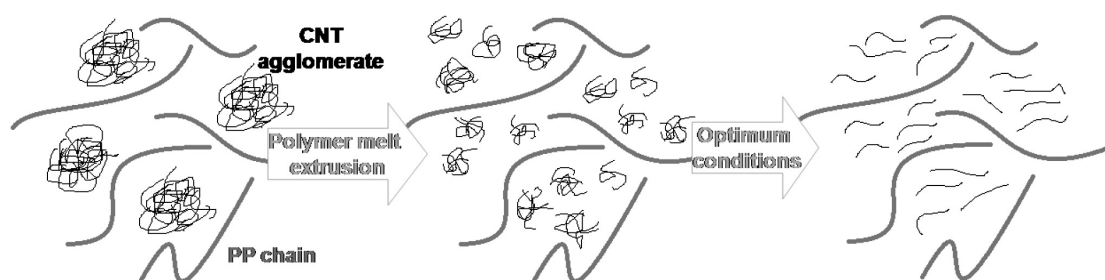
Figure 1: Exfoliated nanocomposite formation during the polymer-melt mixing
