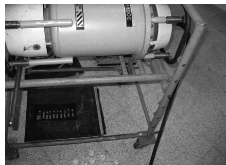
Figure 6: Film, penetrometer, stenciling pattern and beam setting Slika 6: Film, merilec globine penetracije, vzorec šablone, nastavitve snopa
