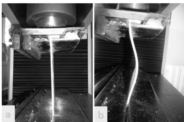
Figure 2: View of the buckling-test process: a) before buckling and b) after buckling
