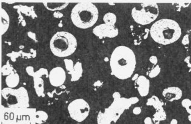
Figure 7: Internal porosity of nearly spherical Cu-Ag alloy-powder particles.
