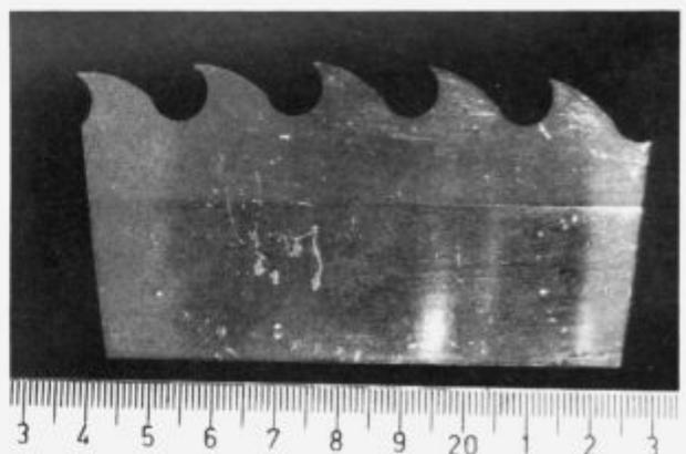
Figure 16: Vacuum brazing of high speed steel (circular saw segments) on the structural steel base.
