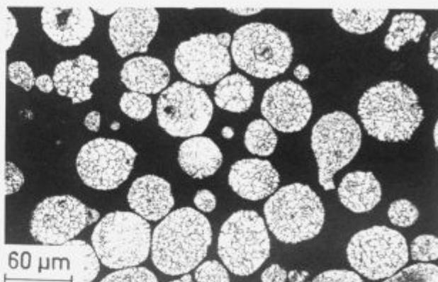
**Figure 4:** Cellular solidification of Cu-2%Ni alloy-powder particle.
