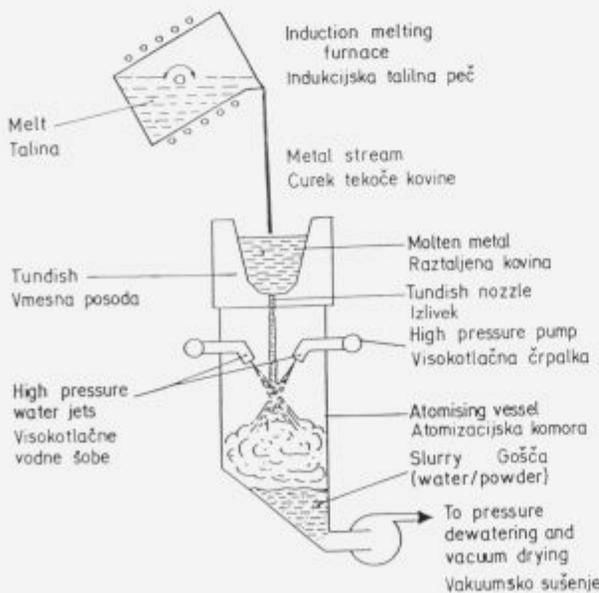
**Figure 2:** Schematic presentation of water atomization<sup>6</sup>
