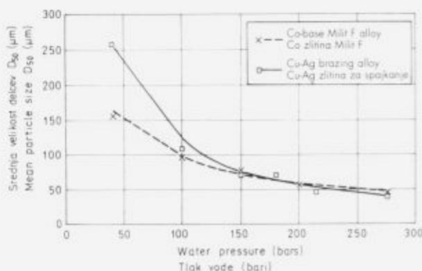
Figure 9: Mean particle size vs. water pressure for Cu-Ag brazing-alloy powder and Co-based welding-alloy powder.
