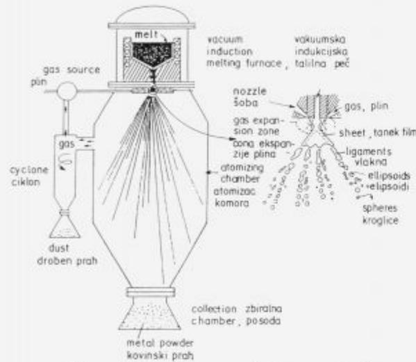
**Figure 1:** Schematic presentation of gas atomizer<sup>4</sup>
