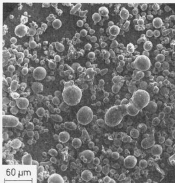
Figure 6: Particle shape of prepared Cu-2%Ni alloy-powder.
