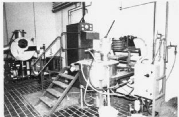
**Figure 3:** PM&RST laboratory at the IMT Ljubljana with water atomizer in the foreground.
