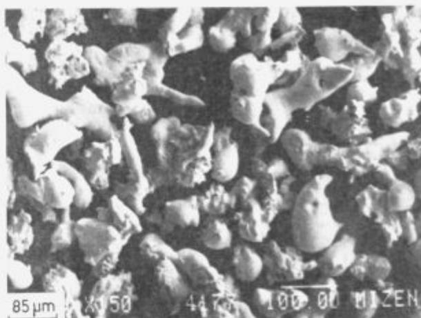
Figure 8: SEM micrograph of Au-Cu water atomized powder with irregularly shaped (tear drop and ligamental) particles.
