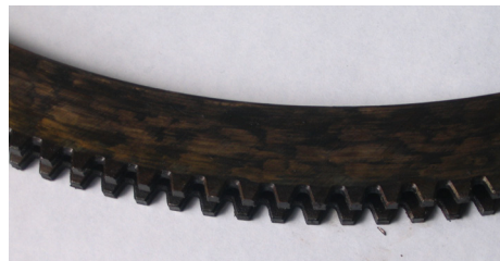
Fig. 9. Traces of the damage on a steel disc after tests
