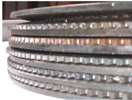
Fig. 8. Deformed package of discs of brake F_5 after tests
