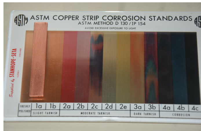
Fig. 7 Determination of corrosiveness to copper for IL-11 17PI045
