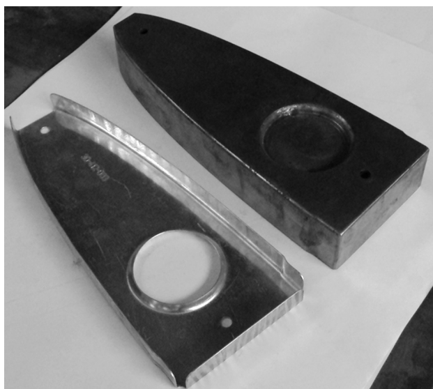
Figure 5: Rib with a lightening hole fabricated by the rubber-pad forming process and the die
