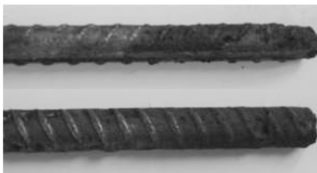
Figure 11: Steel reinforcements cleaned with a Clarke solution Slika 11: Z raztopino Clarke očiščena jeklena armatura
