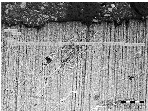
Figure 4: Microstructure of test specimen D99: positive segregations – tempered martensite (dark bands), 4% picral
