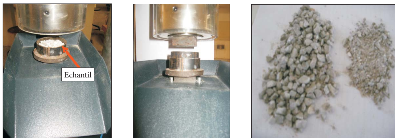
Figure 5. Crushing tests of samples composed of multiple grains.
