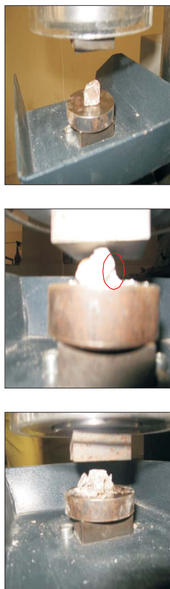
Figure 2. Tests crushing grain by grain.
