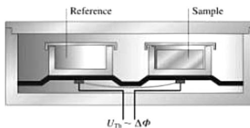
**Figure 5.** Schematic presentation of the heat flux DSC with a disk type measuring system<sup>[12]</sup>
