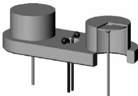
**Figure 9.** Position of the reference sensor: Tzero™ sensor<sup>[17]</sup>
