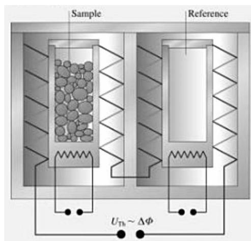
**Figure 6.** The heat flux DSC with a cylinder-type measuring system (Calvet)<sup>[12]</sup>
