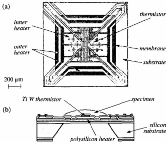
**Figure 4.** Schematic representation of  $\mu$ -DTA: optical micrograph of a membrane with inner and outer polysilicon heaters and central TiW thermistor (a) and schematic cross section of the membrane with melted specimen (b)<sup>[6]</sup>
