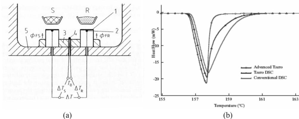
**Figure 8.** The turret type measuring system HF-DSC <sup>[1]</sup> (a) and effect by melting indium<sup>[1, 18]</sup> (b) specimen<sup>[6]</sup>
