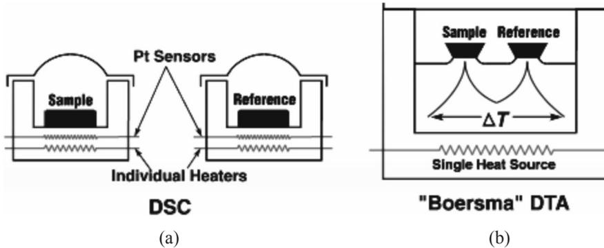
**Figure 2.** Schematic layout of the DSC apparatus: PC-DSC (a) and quantitative (Boersma) DTA or HF-DSC<sup>[3]</sup> (b)
