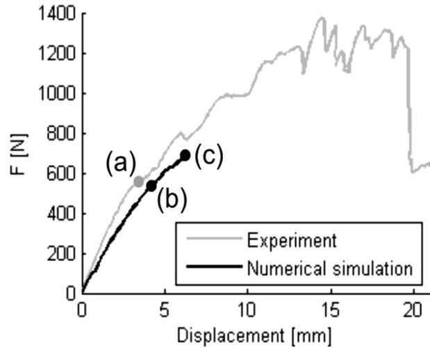
**Figure 4:** Load-displacement diagrams of the experiment and the numerical simulation: a) first failure investigated using experiment, b) first failure investigated using numerical simulation and c) loss of numerical stability
