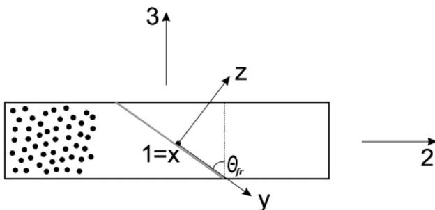
**Figure 1:** Description of the material coordinate system (1, 2, 3) and the crack coordinate system (x, y, z)
