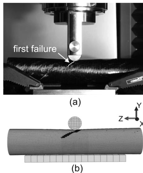
**Figure 5:** Comparison of the position and shape of the first failure investigated using the experiment and the numerical simulation
