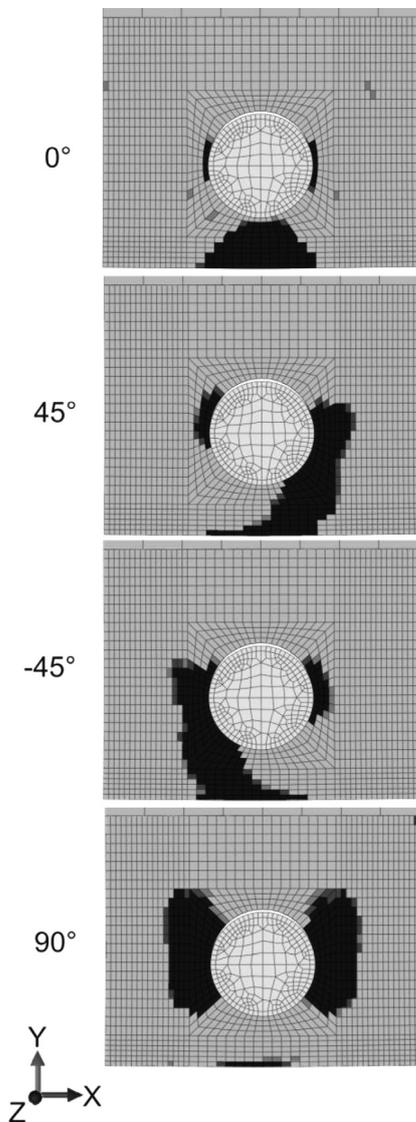
**Figure 3:** Numerical simulation of the final shape of failure in the case of specimens with a shear-out failure mode; different layers displayed
