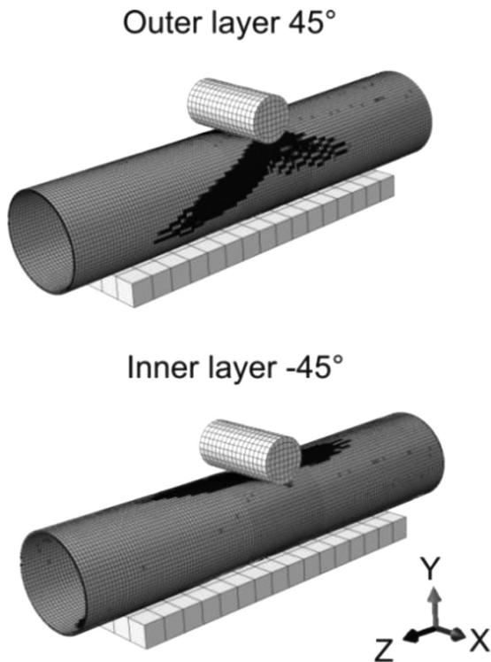
**Figure 6:** Numerical simulation of the shape and the position of failure just before the loss of numerical stability
