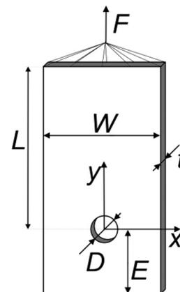
**Figure 2:** Geometric properties of the pin-loaded plate
