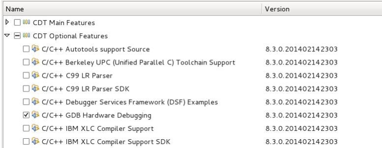
Figure 1.2: Select C/C++ GDB Hardware Debugging plug-in in the *Install* dialog box
