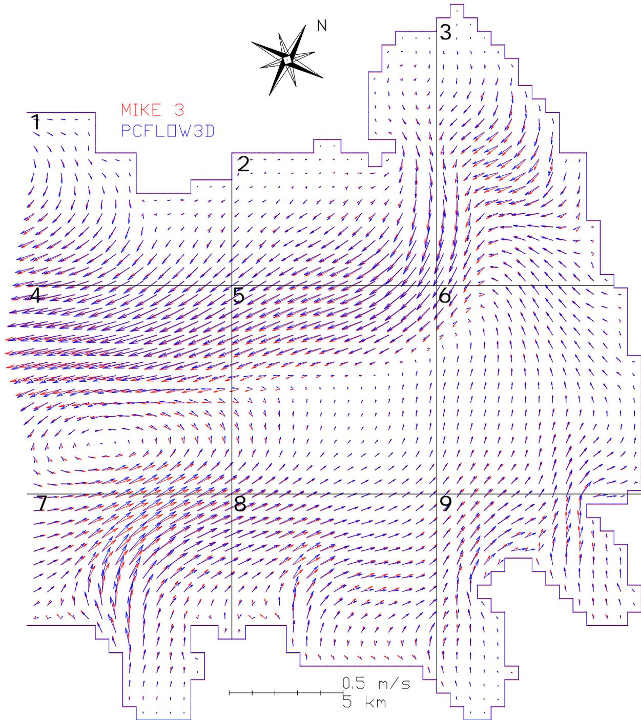
**Figure 1:** Simulation A1 (density-driven flow) – time of simulation 48h (25<sup>th</sup> layer) RMSDN = 0.195 (excellent agreement).
