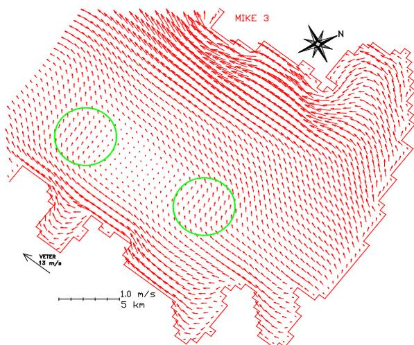
**Figure 7:** Model MIKE3 – winter simulation with bora wind, surface layer.
