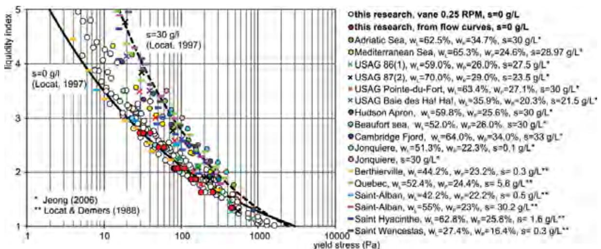
Figure 7. Yield stress and liquidity index of the investigated marine sediments in comparison with the literature data [9, 27, 37].
