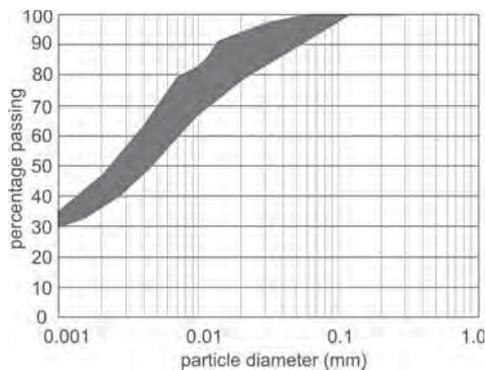
**Figure 2.** Representative area of grain size distribution.
