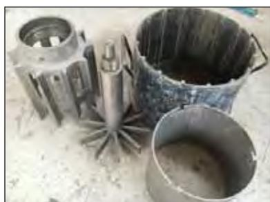
Figure 4. ConTec Viscometer 5.
