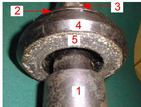
Fig.10. Photograph of asphalt holder: shaft (1), pressing plate (2), fastening screw (3), rubbing ring (4), asphalt (5)
