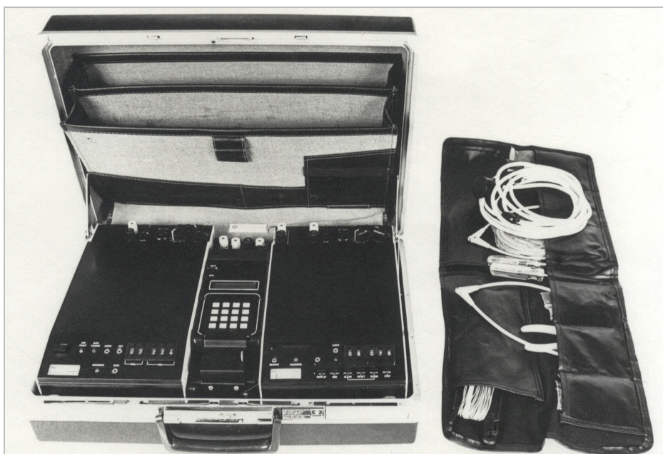
The portable Racial radio station was built into a standard Samsonite briefcase (SI AS 1931, t. e. 225, Sistem agenturnih vez Racial, 30. 6. 1983)
