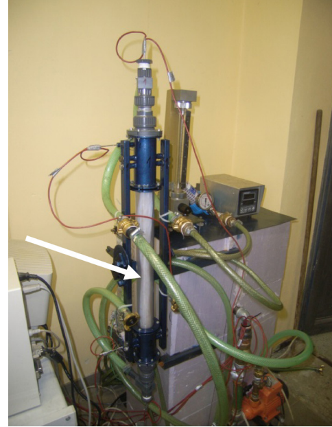
Fig. 10. Heat exchanger with tangential inlet and sliding head
