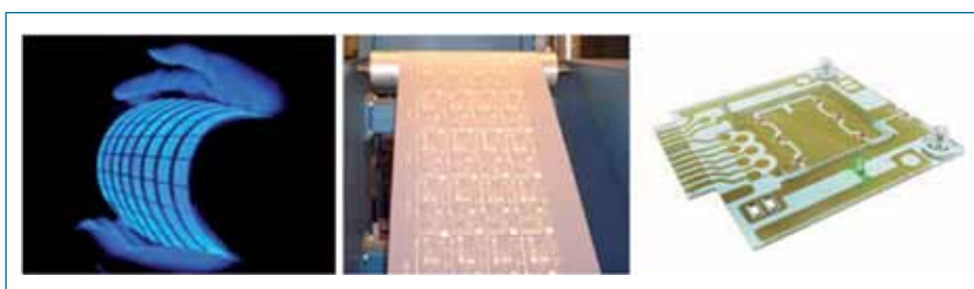
Slika 1: Stopnje tiskane elektronike: (a) waferska, (b) tiskana in (c) hibridna stopnja [1] Figure 1: Levels of printed electronics technology: (a) wafer, (b) printed and (c) hybrid [1]
