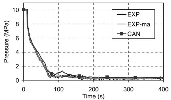
Figure 4. Header 7 pressure for the RD-14M test.
