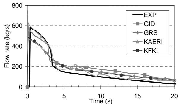
Figure 2. Break flow rate for the LOFT L2-5-test.
