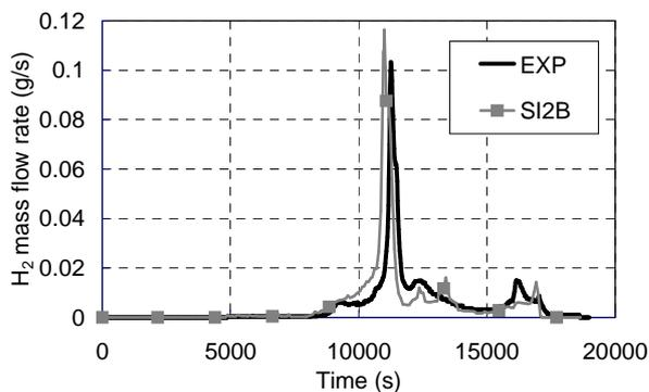
Figure 3. H<sub>2</sub> mass flow rate for the Phebus FPT1 test.
