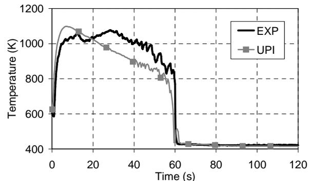
Figure 1. Rod surface temperature for the LOFT L2-5-test.
