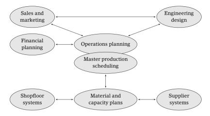
FIGURE 3 Production Planning System Supporting MTO Environment
