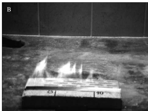
Figure 2. Combustion front propagation determination for hexamethylenetetramine: A) initial point, B) final point
