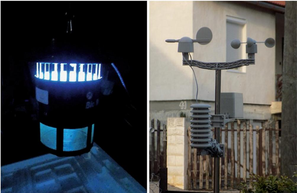
**Fig. 2.** Operating Bio Mosquito Trap (left) and the Velleman WS1080<sup>TM</sup> meteorological station (right).
