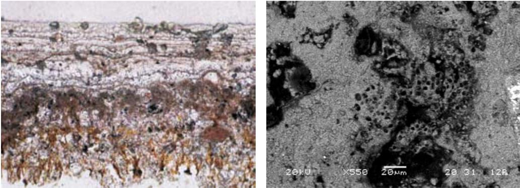
**Figure 5.** a) Filamentous algae and cyanobacteria under laminated calcite crust. Sample RO69, transmitted light, parallel polars; b) Effect of microbial activity in the form of biopitting, sample RO70, SEM, SE
