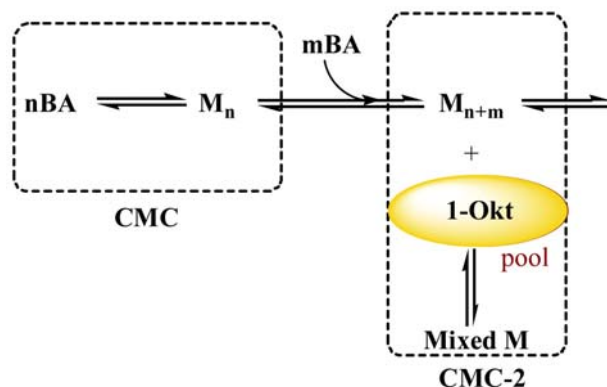
Figure 5. Process of aggregation of Na-12-MKC in D_2O solution saturated with 1-octanol. BA – monomer of Na-12-MKC, M – micelle of Na-12-MKC, 1-Okt – 1-octanol, Mixed M – mixed micelle of Na-12-MKC and 1-octanol.
