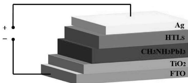
**Figure 1:** Schematic representation of a perovskite solar cell
