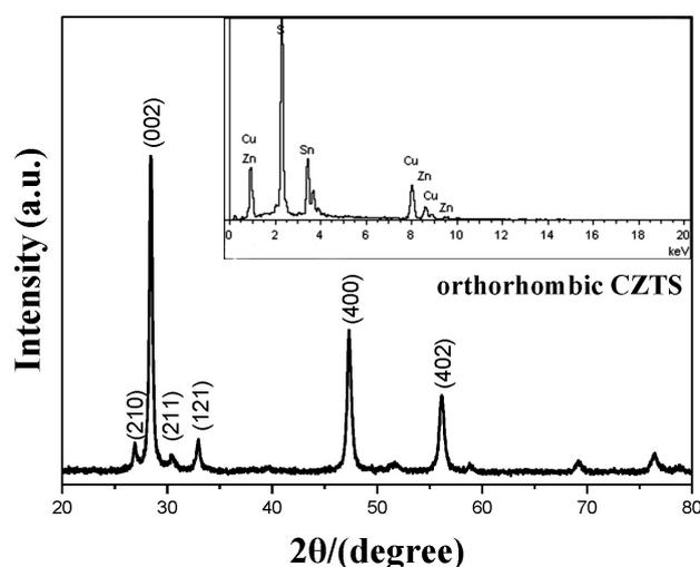
**Figure 2:** XRD pattern and EDS image of CZTS NPs
