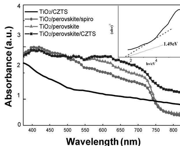
**Figure 3:** UV-vis absorption spectra for: a)  $\text{TiO}_2$ /perovskite/CZTS, b)  $\text{TiO}_2$ /perovskite, c)  $\text{TiO}_2$ /perovskite/spiro-OMeTAD, d)  $\text{TiO}_2$ /CZTS films and band gap of CZTS
