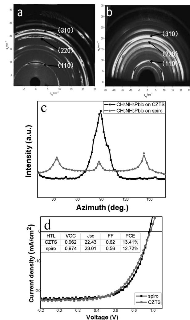
**Figure 4:** GIXRD pattern of CH<sub>3</sub>NH<sub>3</sub>PbI<sub>3</sub> deposited on: a) CZTS, b) spiro-OMeTAD, c) the corresponding radially integrated intensity plots along the ring at  $q \approx 10 \text{ nm}^{-1}$  for the two films derived from a) and b), respectively, d) J-V characteristics of the champion perovskite solar cells using spiro-OMeTAD and CZTS as HTLs
