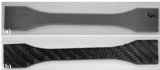
Figure 1: a) glass-fiber and b) carbon-fiber-PR-based composites; specimens for tensile tests
