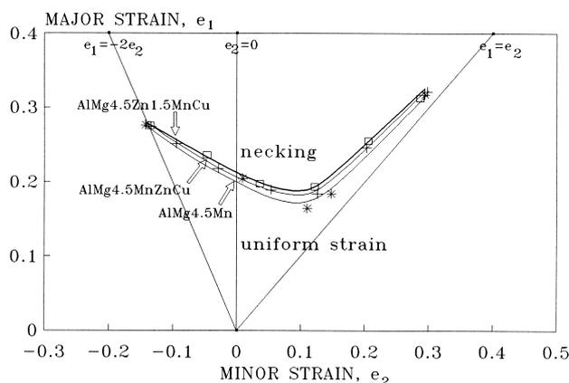
**Figure 1:** Forming-limit curves of the investigated alloys. The *e*<sub>1</sub> and *e*<sub>2</sub> are the true strains (major and minor strain in the plane of the sheet).
