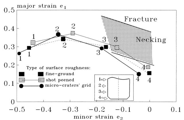
**Figure 4:** Influence of the surface roughness on the strains along the wall of the deep-drawn cup of AlMg4.5Zn1.5MnCu sheet
