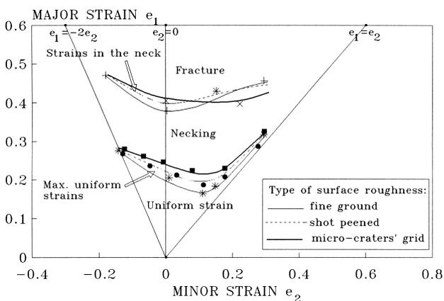
**Figure 3:** Influence of the surface-roughness type on the forming limit curves of AlMg4.5Zn1.5MnCu sheets
