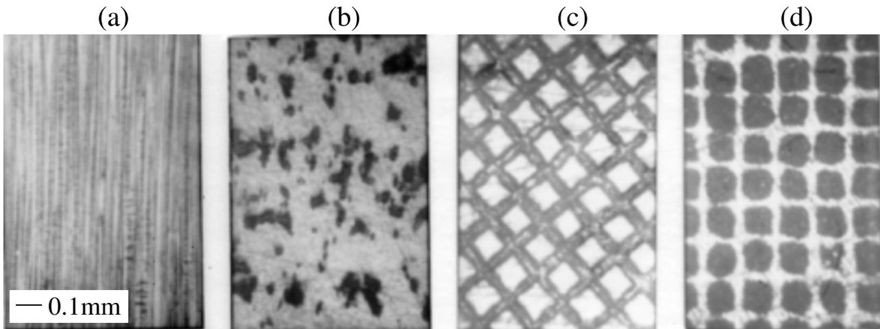
**Figure 2:** Surface roughness of sheets, produced by: a) rolling with fine-ground rolls; b) shot peening; c) photo etching of micro-channels' grid; d) photo etching of micro-craters' grid
