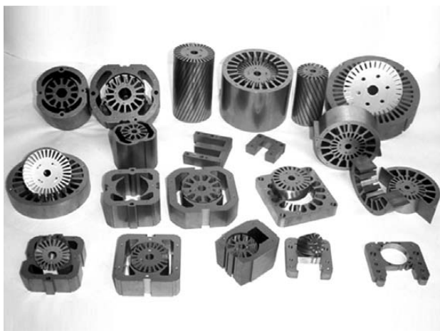
Figure 2: Some parts manufactured with the WEDM process 7
