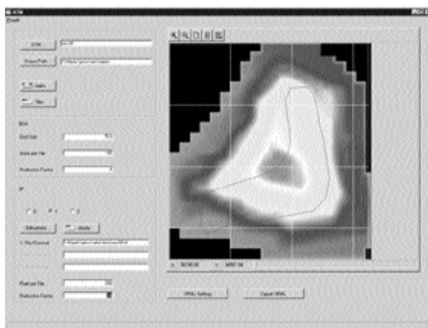
Figure 2: User interface of ATM showing coded DTM and defined flight path.
