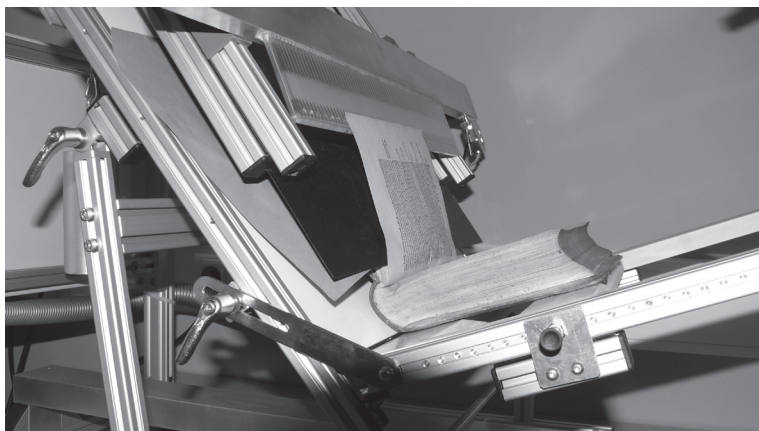
Picture 6: Detail of the setup showing that every single leaf of the book will be held flat in a certain position by a vacuum bar.
