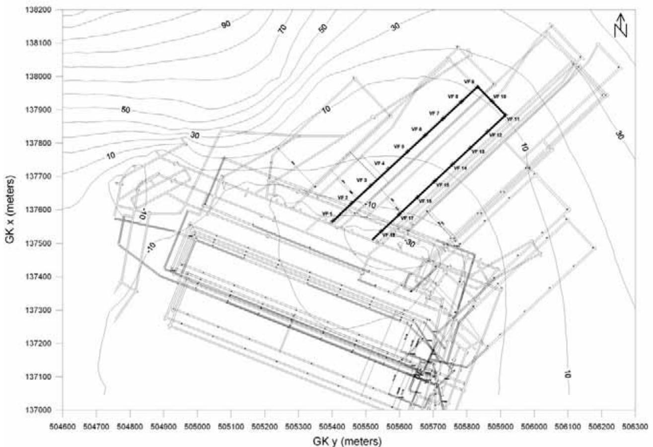
Figure 5. Groundwater-level contour map for the water-bearing sands P11 & P12 in 2007 (with north to the top). The underground vertical pumping wells are marked with the labels VF (black points).
