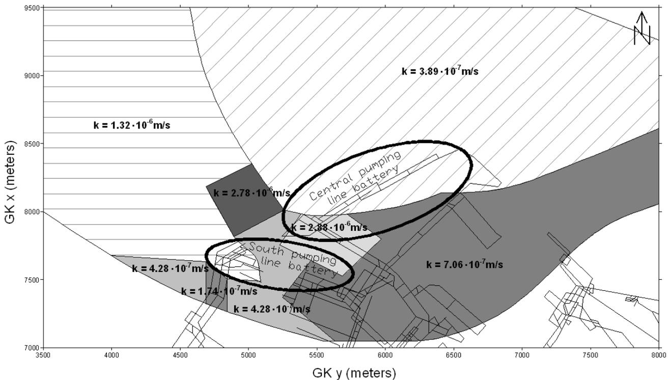
**Figure 6.** Map of the hydraulic conductivity zones of the modelled P11 sands deduced from a series of pumping tests. The zones were defined in one of the previous models in the ModFlow 4.2 FDM (North is orientated vertically).
