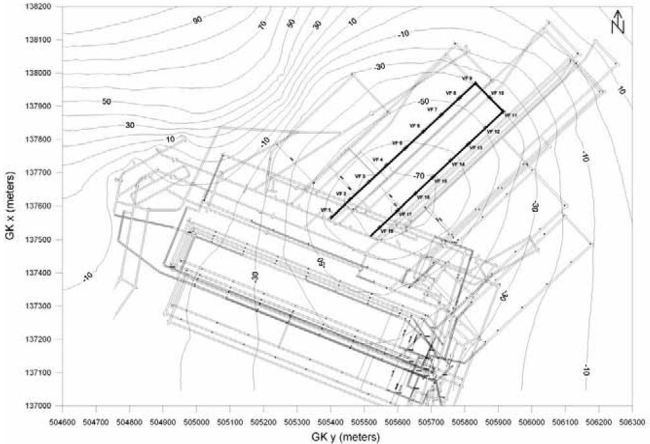
**Figure 8.** Predicted groundwater-table depression in 2012 after 230 days of mining operations on a longwall face. All the "drive-in" filters are in operation. (North is vertically orientated).
