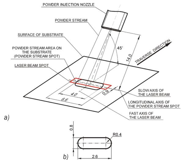
**Fig. 3.** Diagram showing a) the alignment of the powder injection nozzle relative to the laser beam spot, and b) the geometry of the powder injection nozzle opening used
