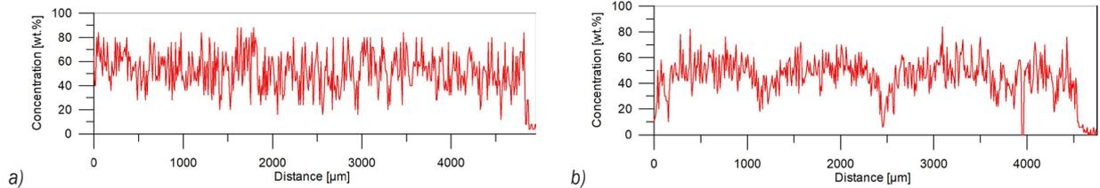
**Fig. 5.** Chromium concentration profiles on the cross-section of the SB no.: a) C3; b) C4. Results from SEM/EDS line-scans analysis collected along line parallel to the bead surfaces at 350  $\mu\text{m}$  depth
