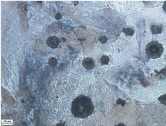
**Fig. 1.** Microstructure of the used DCI grade EN-GJS-700-2
