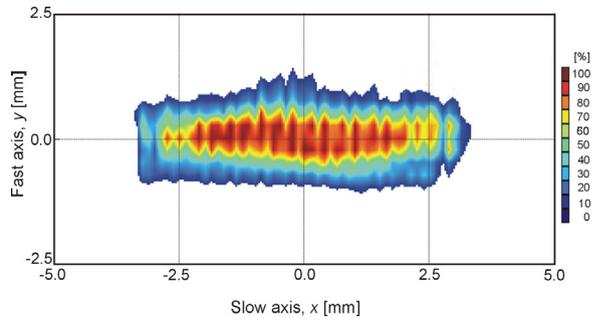
**Fig. 2.** 2D beam profile of the used HPDD laser in the focal plane
