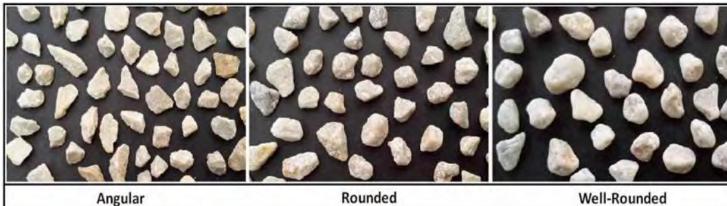
**Figure 3.** Pictures of soil with three different roundness.
