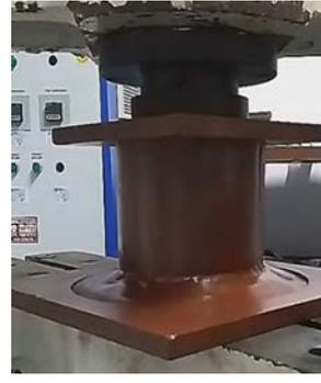
Fig. 14. PPS specimen after collapse
