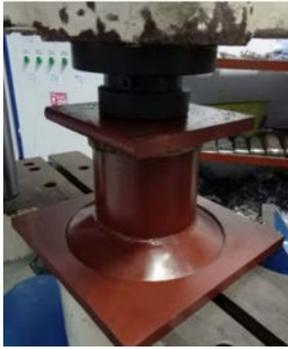
Fig. 13. PPS specimen before collapse
