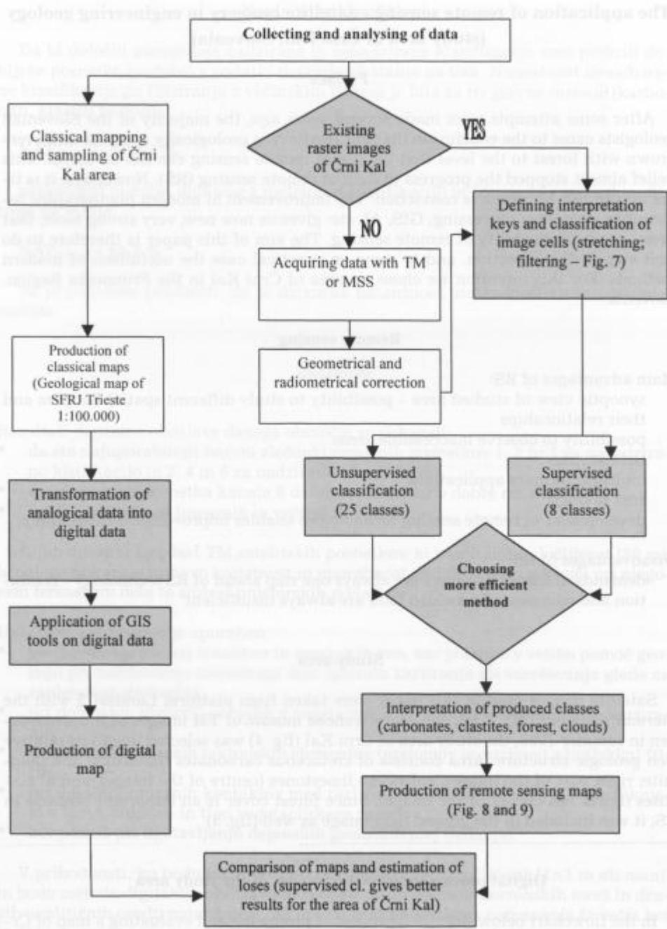
Fig. 10. Process of producing and evaluating a RS map of studied area
