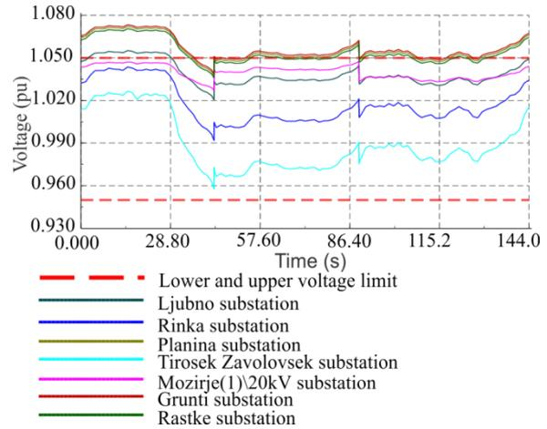
Figure 7: Classical voltage control – MP voltages.
