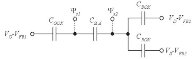
Fig. 3. Equivalent capacitive circuit of the VFD SONFET in the subthreshold region.
