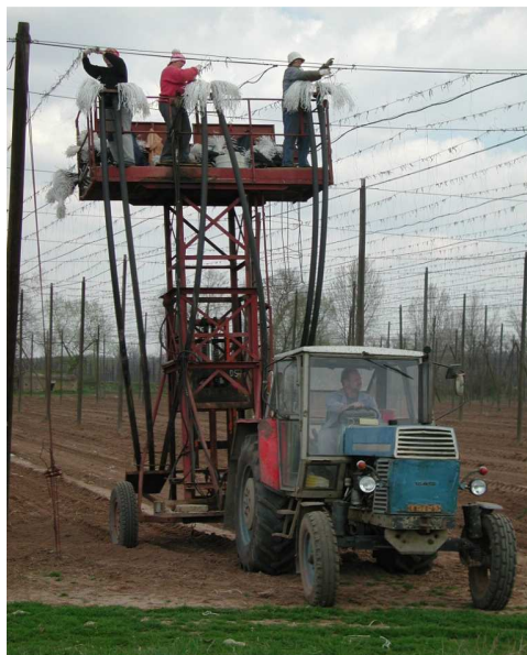
Figure 3: Tractor-drawn platform used for stringing
