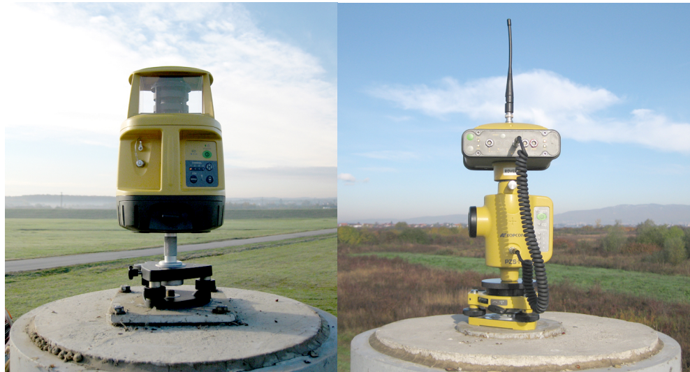
Fig. 2: (a) PZL-1 laser transmitter and (b) PZS-1 sensor connected to GNSS rover receiver.
