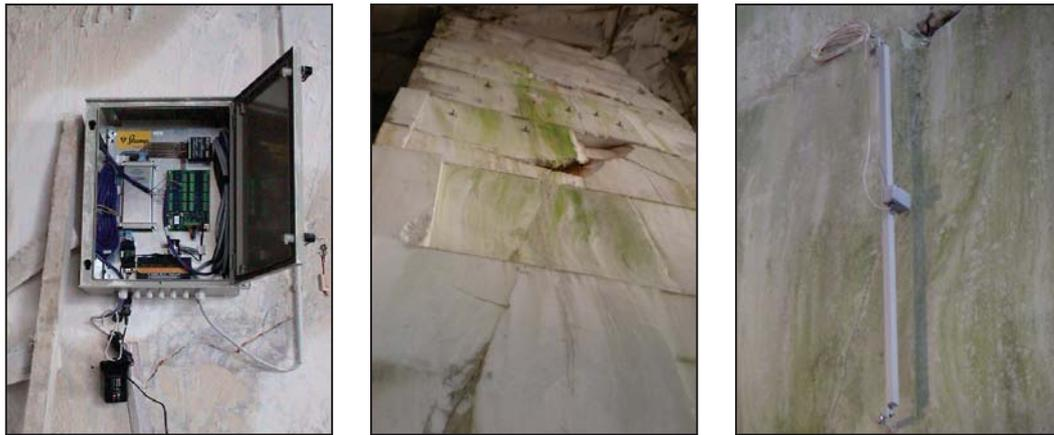
Figure 7. Datalogger (left) with vertical EL beam gauge (right) installation on the high safety pillar VS3 stabilized with anchors (middle) in Lipica II. quarry.
