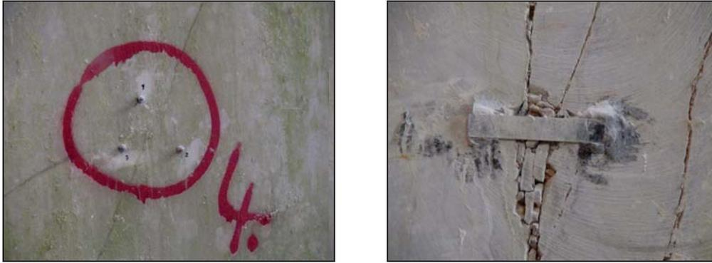
Figure 1. 3 screw open fissures displacement meter (left) and glass fissures displacement meter/seal (right) for visual monitoring of underground structures stability in Lipica II. quarry.
