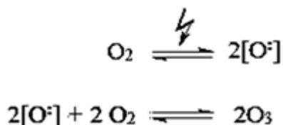
Ozone production varies depending on oxygen concentration in feed gas, dielectric material property, discharge gap, current frequency and voltage. The electrodes are often cooled to remove excess heat and prevent the decomposition of ozone generated (Oner & Demirci, 2016; Pandiselvam et al., 2017).
