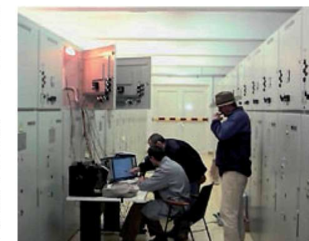
Figure 4: Electromagnetic compatibility testing inside a power substation
