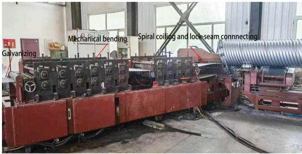
**Figure 15:** Production line of roll-forming process
