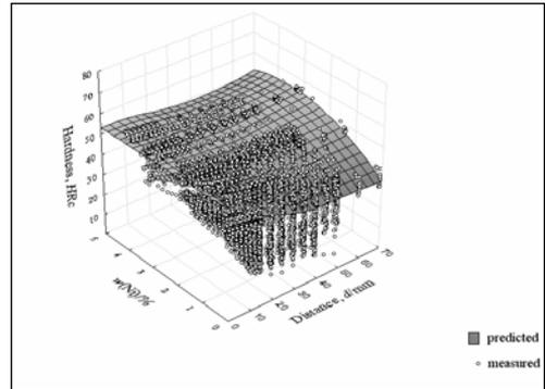
**Figure 4.** Dependence of hardness (measured – markers and predicted – area) upon amount of nickel and distance
