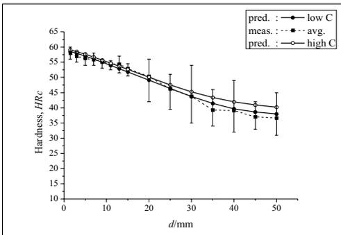
**Figure 9.** Measured and predicted hardness profile for steel grade 42CrMoS<sub>4</sub>
